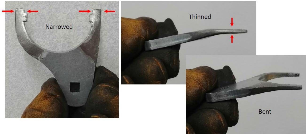
Figure 22. Crows Foot Adapter Adjuster Modified for WJ Knuckles
