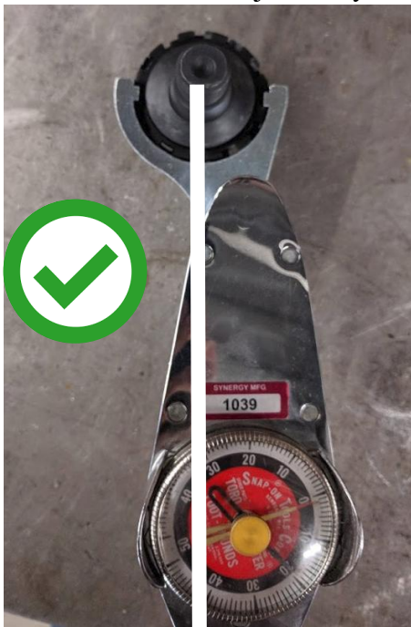
Figure 20. Correct Wrench Orientation
