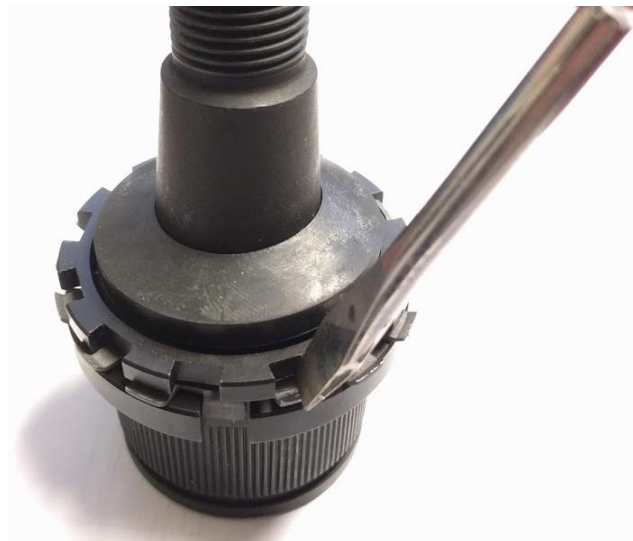
Figure 19. Bending Locking Tabs Back
