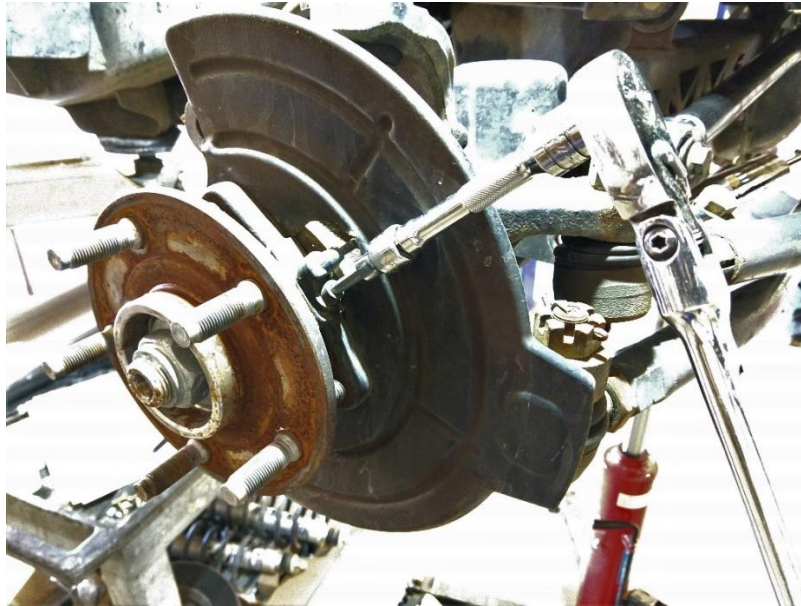
Figure 4. ABS Sensor in Knuckle
