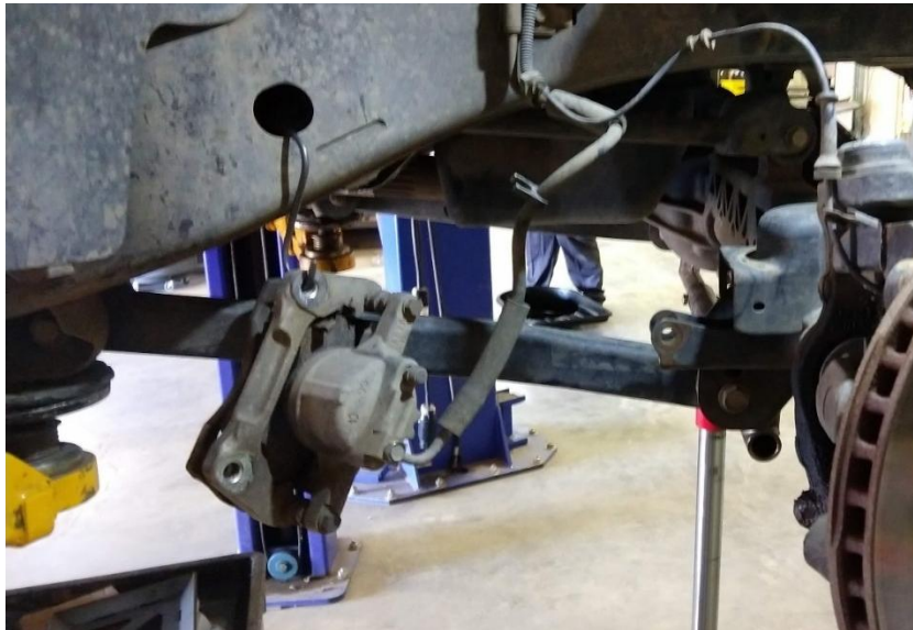
Figure 3. Hanging Brake Caliper
