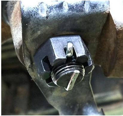
Figure 14. Cotter Pin Installed
