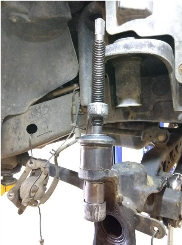
Figure 8. Pressing Out Upper Ball Joint
