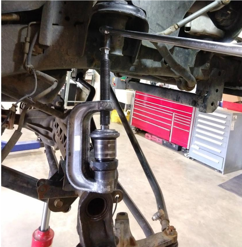
Figure 12. Pressing the Upper Ball Joint into Housing
