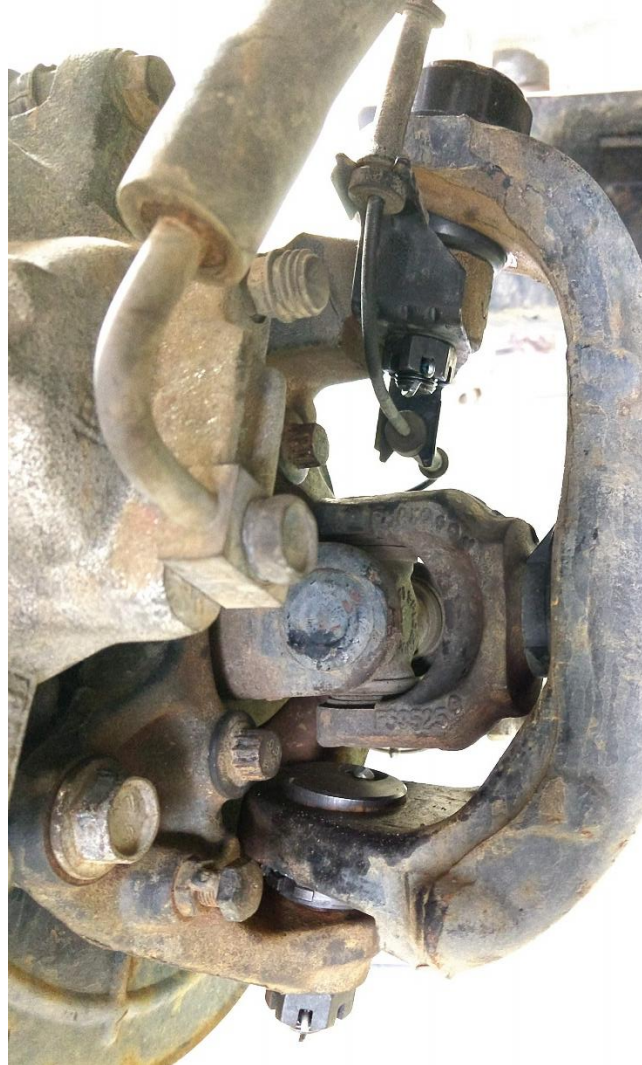
Figure 17. Finished Ball Joint Installation
