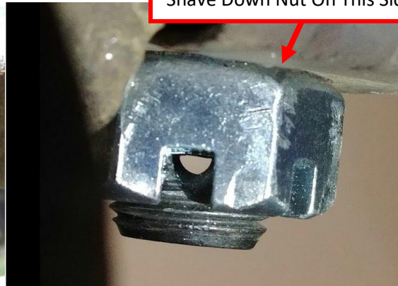
Figure 15. WJ Knuckle Cotter Pin Alignment
