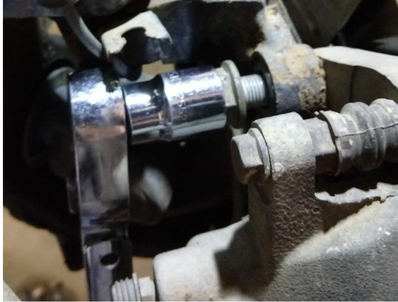
Figure 2. Removing Brake Caliper Carrier Bolts
