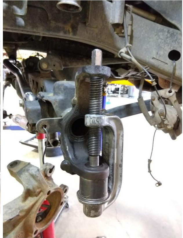
Figure 9. Pressing Out Lower Ball Joint
