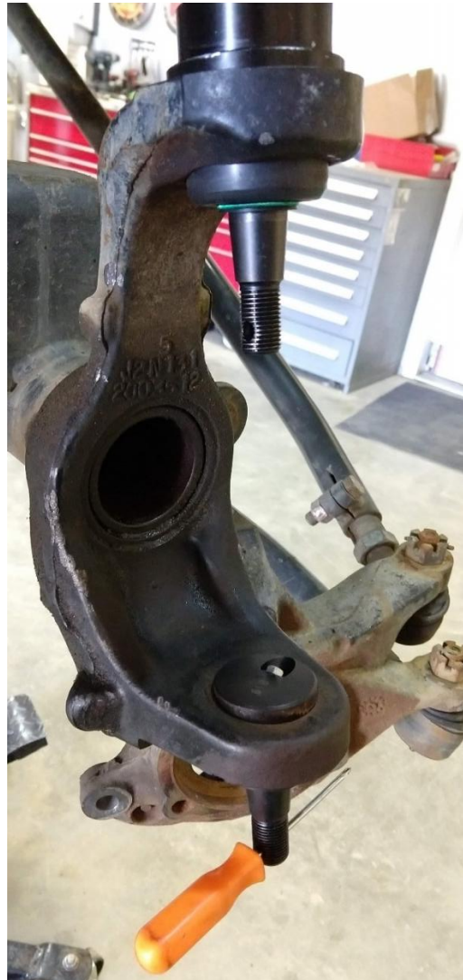
Figure 13. Cotter Pins Aligned Front to Back
