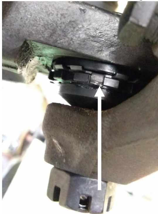
Figure 16. Tab Bent Into Cap
