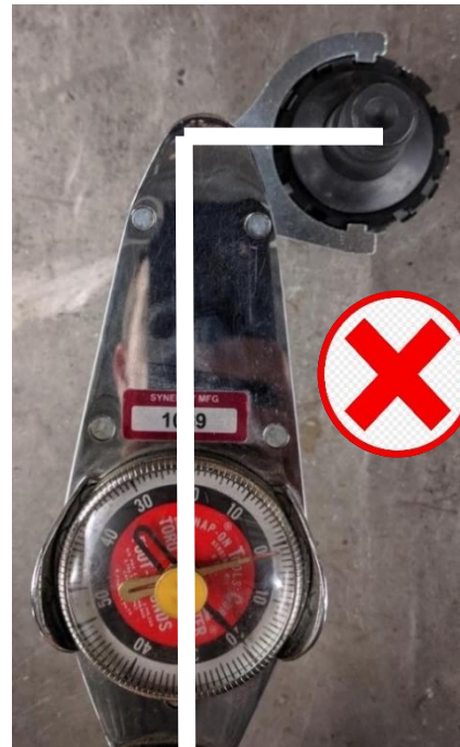
Figure 21. Incorrect Wrench Orientation
