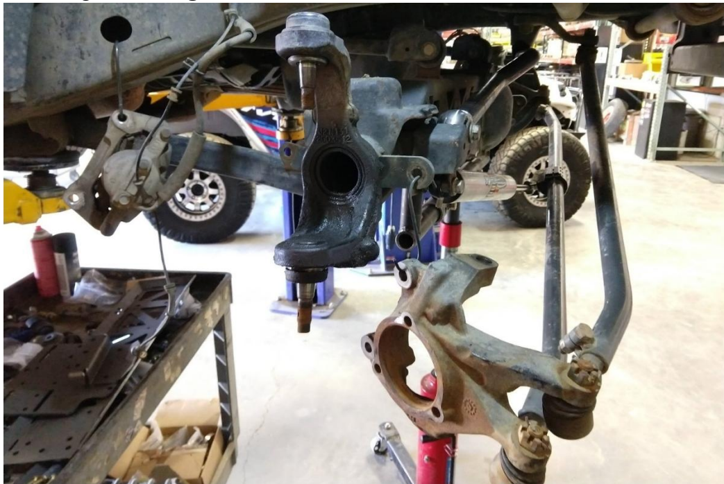
Figure 7. Knuckle Removed, Hanging from Axle Housing
