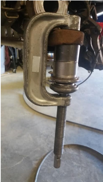
Figure 8. Pressing Out Lower Ball Joint
