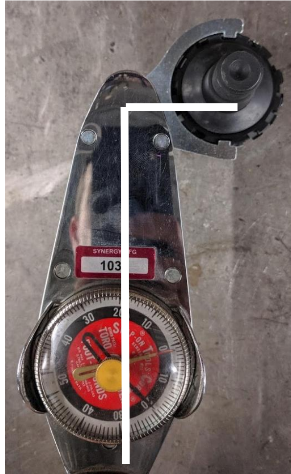
Figure 20. Incorrect Wrench Orientation
