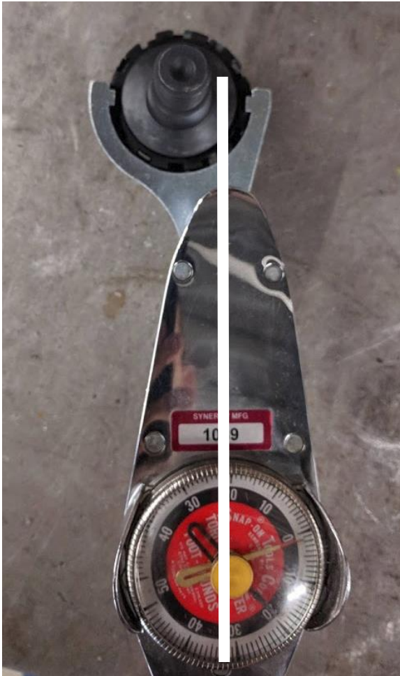
Figure 19. Correct Wrench Orientation
