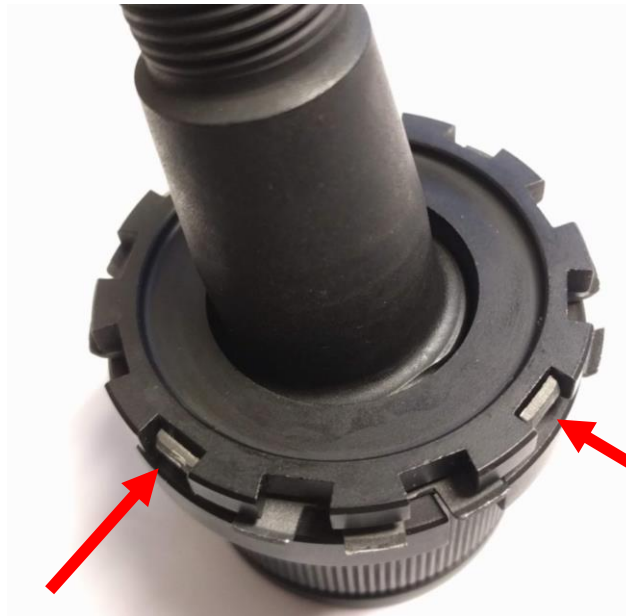
Figure 15. Tabs Bent Into the Cap
