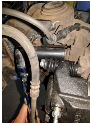
Figure 2. Removing Brake Caliper Carrier Bolts
