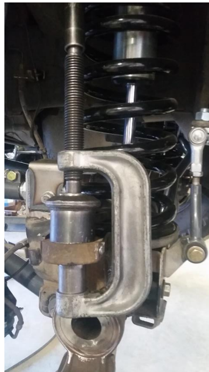
Figure 9. Pressing Out Upper Ball Joint
