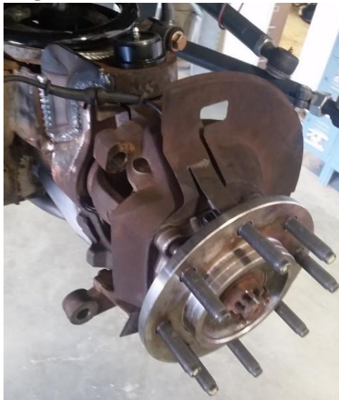
Figure 16. Backing Plates, Hubs and ABS Lines Re-Installed
