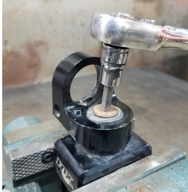
Figure 2. Removing the Clamp Retaining Screw
