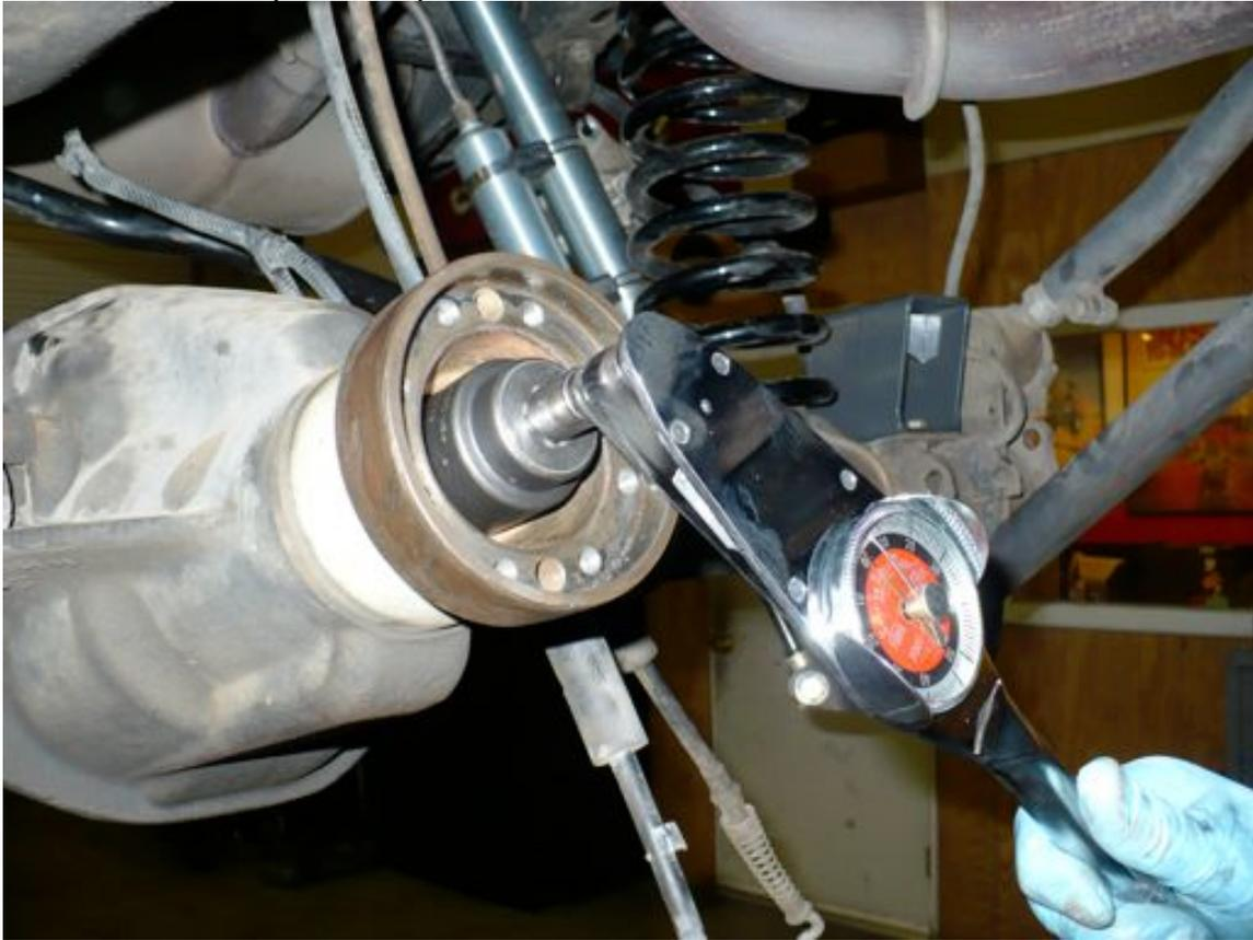
5. Remove the T-case yoke nut and yoke. An air impact works well. Sometimes a puller is needed to remove the yoke.
