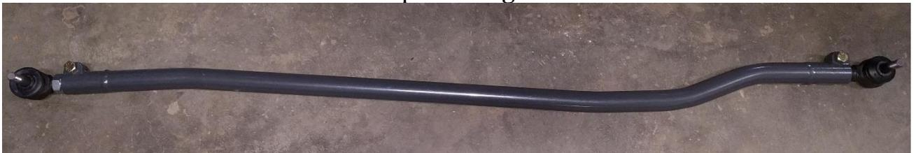
**Figure 4. Synergy MFG Tie Rod Shown From Above**
